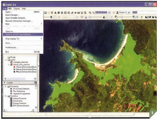
▲ FIGURE 3 ENVI EX includes automated workflows for detecting change over time using imagery taken at different times or with different sensors. In this case, ENVI EX is able to easily identify and export areas with significant changes in vegetation both from manmade features (the road in the lower right) and natural activity (the tsunami destruction of shoreline). These results can easily be exported to a geodatabase for further analysis and map composition.
